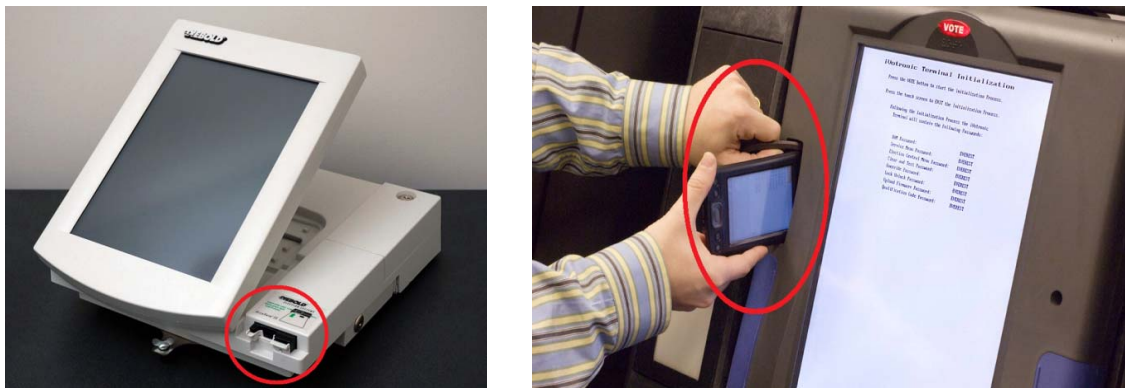
Figure 12: Exposed Removable Media Slots on DREs (Feldman, Halderman and Felten 2007, 1, McDaniel, et al. 2007, 66)
