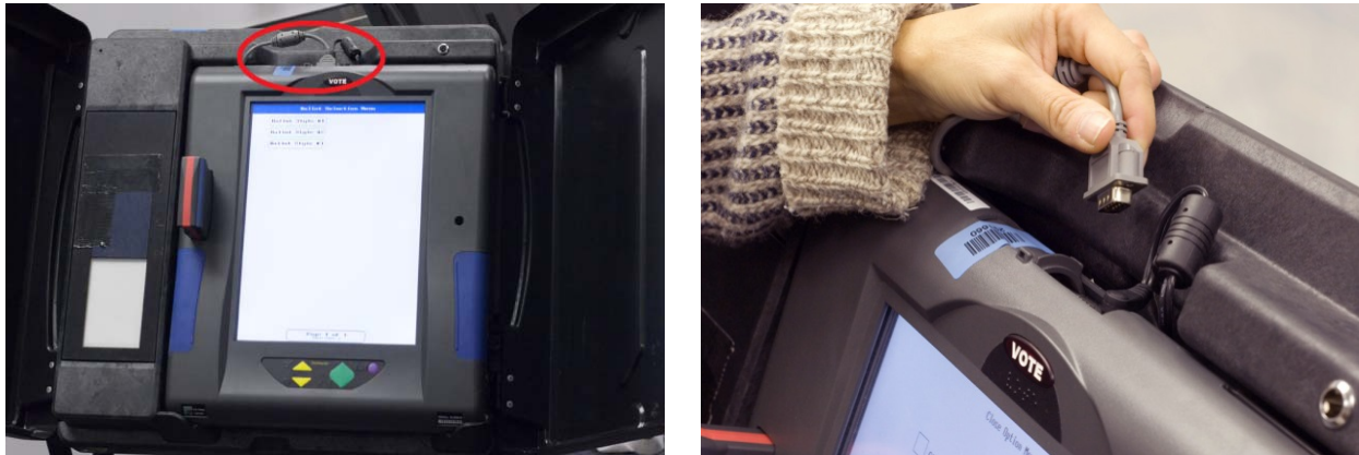
Figure 13: Exposed VVPT Connections (McDaniel, et al. 2007, 46,72)
