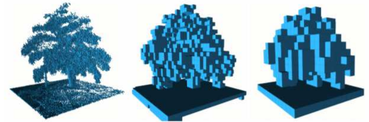
Fig. 3 By limiting the depth of a query, multiple resolutions of the same map can be obtained at any time. Occupied voxels are displayed in resolutions 0.08 m, 0.64 , and 1.28 m.
